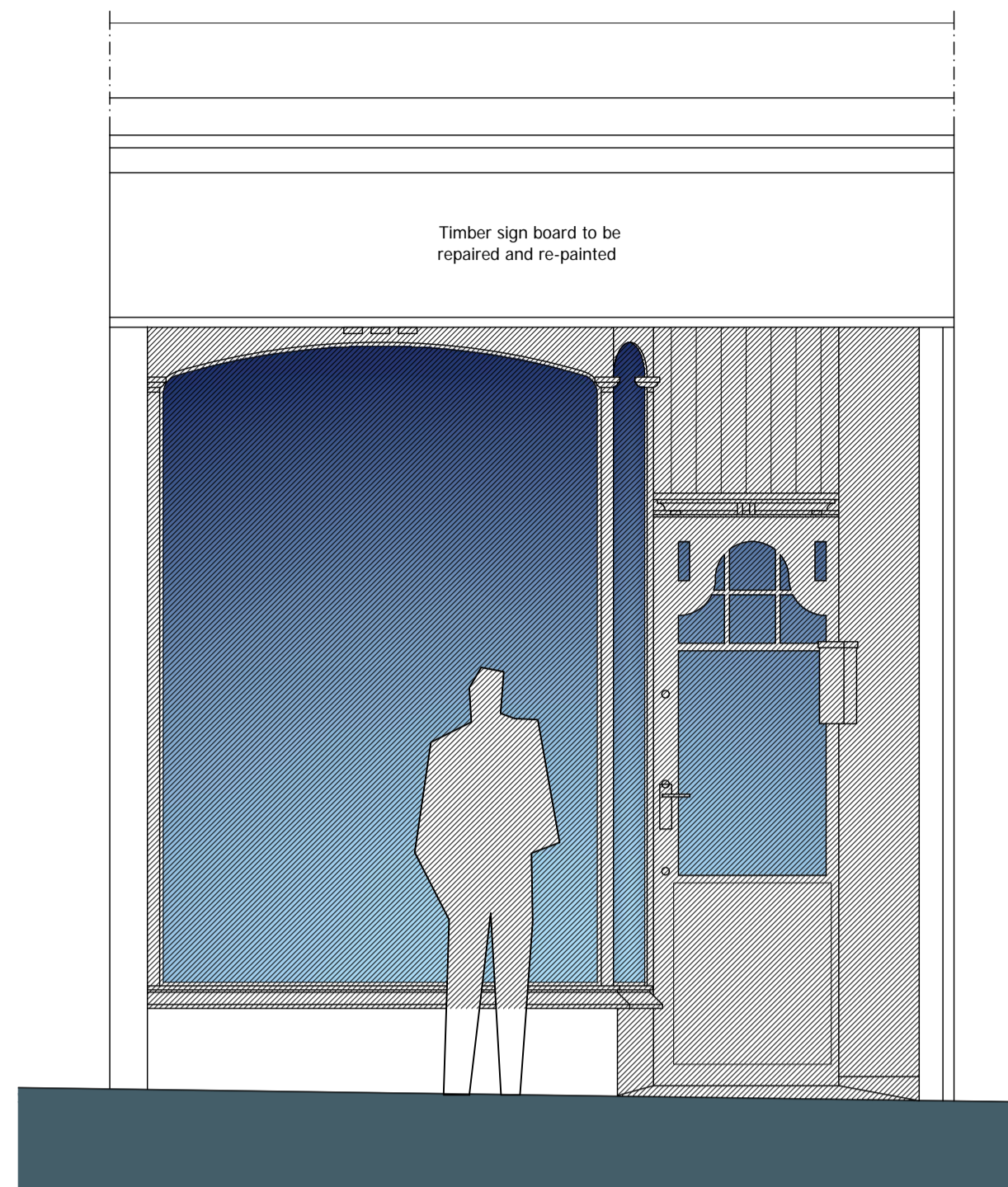
ELEVATION TO KEMPOCK STREET AS EXISTING
